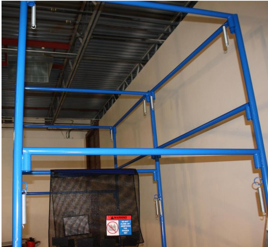
**Step 16:** Prepare each housing – part #63L (left) and #63R (right) – and find the upper loops for each. Begin by attaching the springs to the top of the structure.
