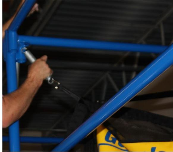
Attach the housing to the loops. Use the spring tool to stretch the springs if needed. Start with from top and move down. Repeat for the other housing.
