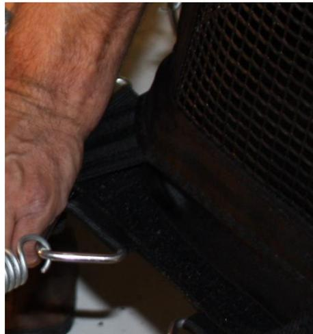
**Step 22:** Attach the left and right housings at the top. Pass the Velcro strap of the left housing through the metal buckle at the top of the right housing. Pull to tighten.
